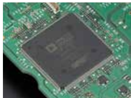
For sub IF DSP, every kind of signal processing ADSP-21369 clock @260 MHz
