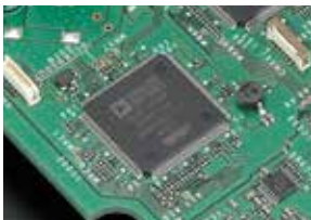
For main IF DSP, transmission unit ADSP-21363 clock @333 MHz
